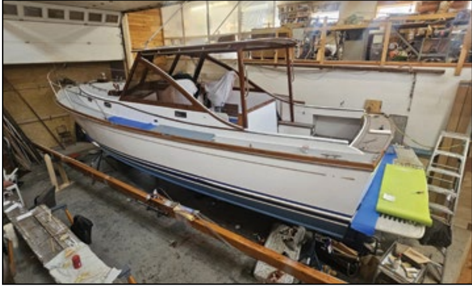
This is an Able 34 at Shop to Shore in South Bristol. She had a complete make over with changes to the windshield and house. She was now getting her varnish redone.
