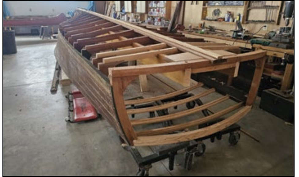
The 1924 Chris Craft in at Woodman Boat Works in Kennebunkport has been turned over so they can put a new bottom on her.
