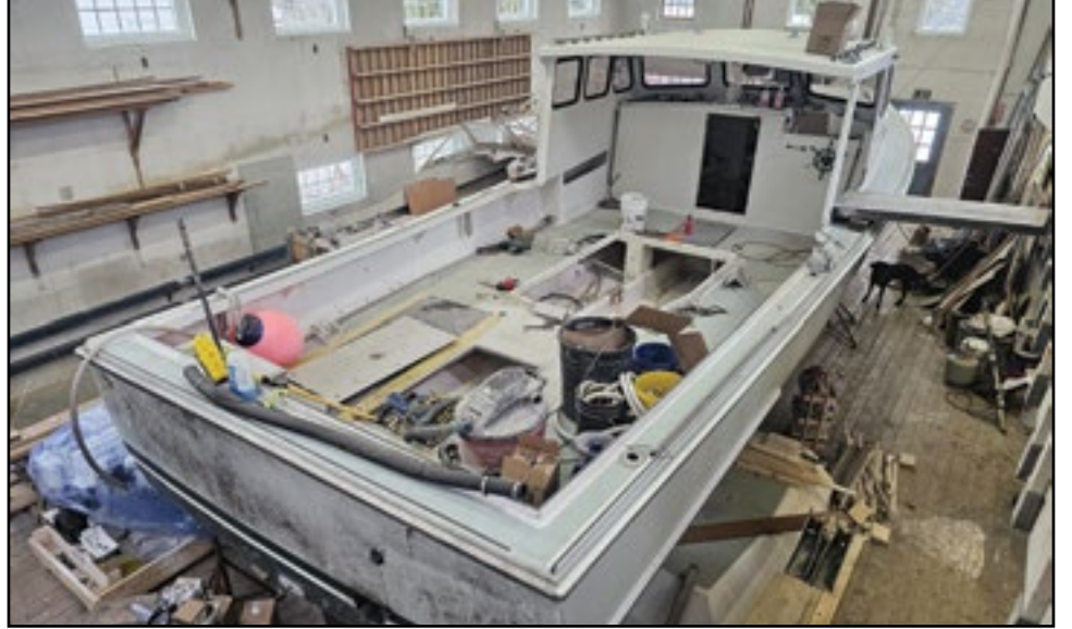
This is a power boat in to be repowered at Finestkind Boat Yard in Harpswell.
