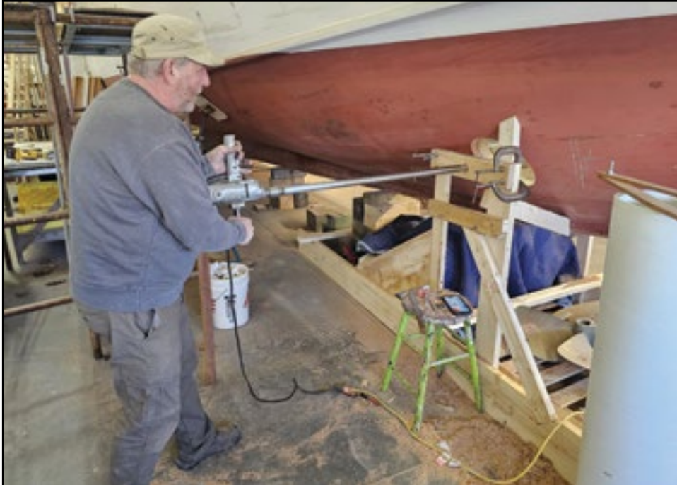
Richard Stanley drilling out a bow thruster at Yankee Marina in Yarmouth.
