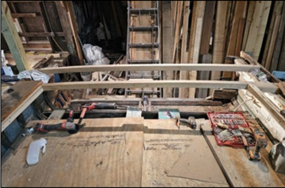
This is a view of the stern of the 28-foot lobster boat/racer CHRISTOPHER, built by Mariner and Isaac Beal in 1976, and owned by Isaac Beal. The transom had some pieces that needed to be replaced. So, the transom was removed and is in the process of being rebuilt.
