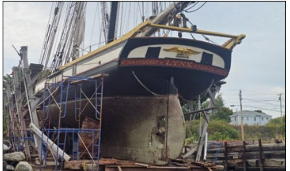
The replica privateer LYNX hauled up on the railway at Northend Shipyard in Rockland.
