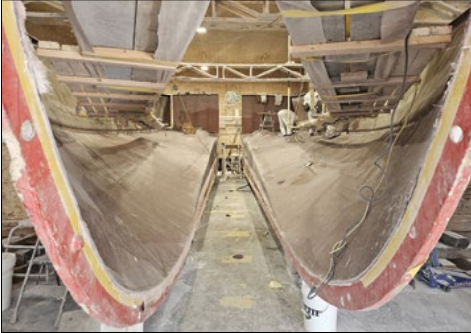
A 50-foot hull being layed up at Wesmac in Surry. The workers are altering the hull for twin Caterpillar diesel engines.
