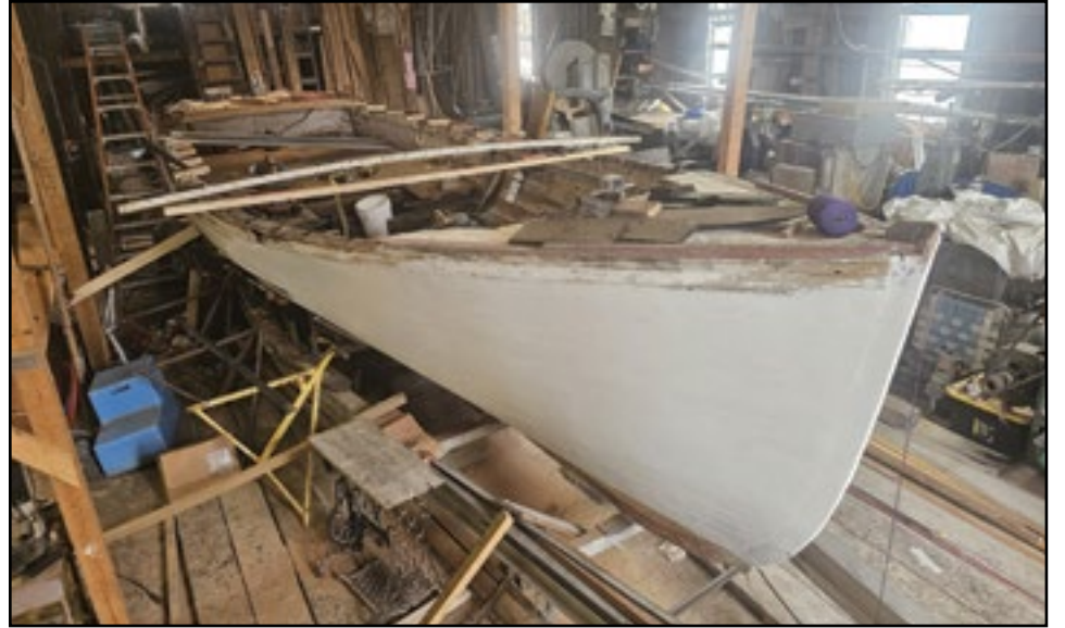
This is Isaac Beal's CHRISTOPHER, a 26-footer that he and his father built and launched in 1976. Note the side deck framing, which Isaac is currently working on.
