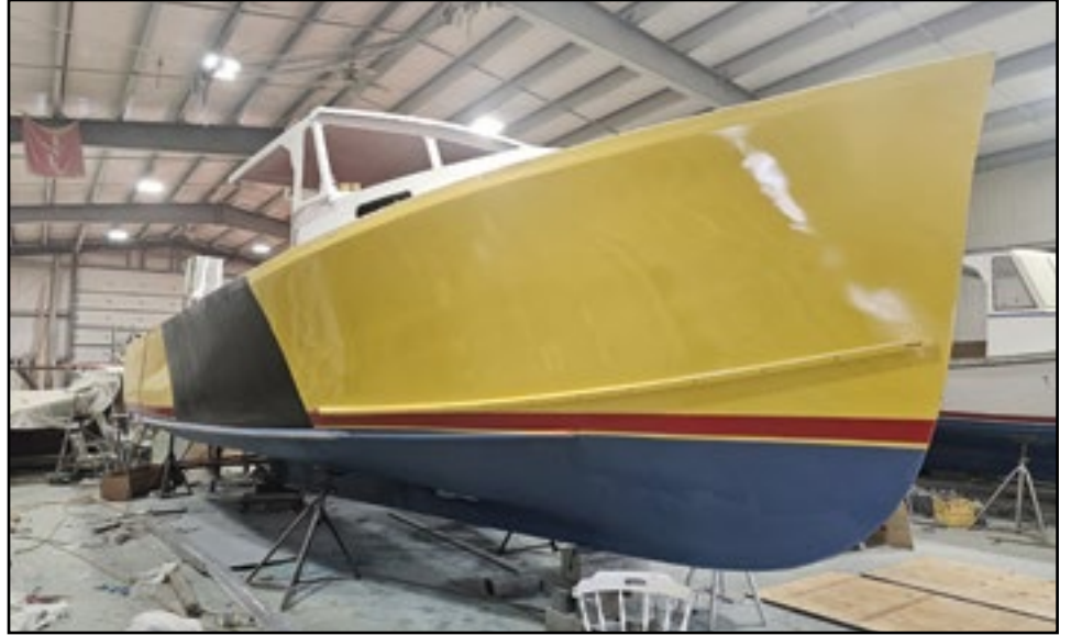
This is a Repco 37, which has been widened by Jermev Beal at Wayne Beal's Boat Shop in Jonesport. She also got a new coat of paint and should be done and out the door in February.
