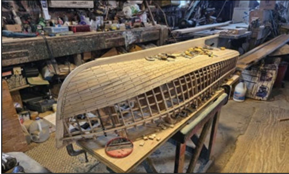
Boatbuilder Willis Beal of Beals Island is back in the shop. He is making another 63-inch model of a lobster boat, the same design as the one he finished last year. This one is for his brother Robert.
