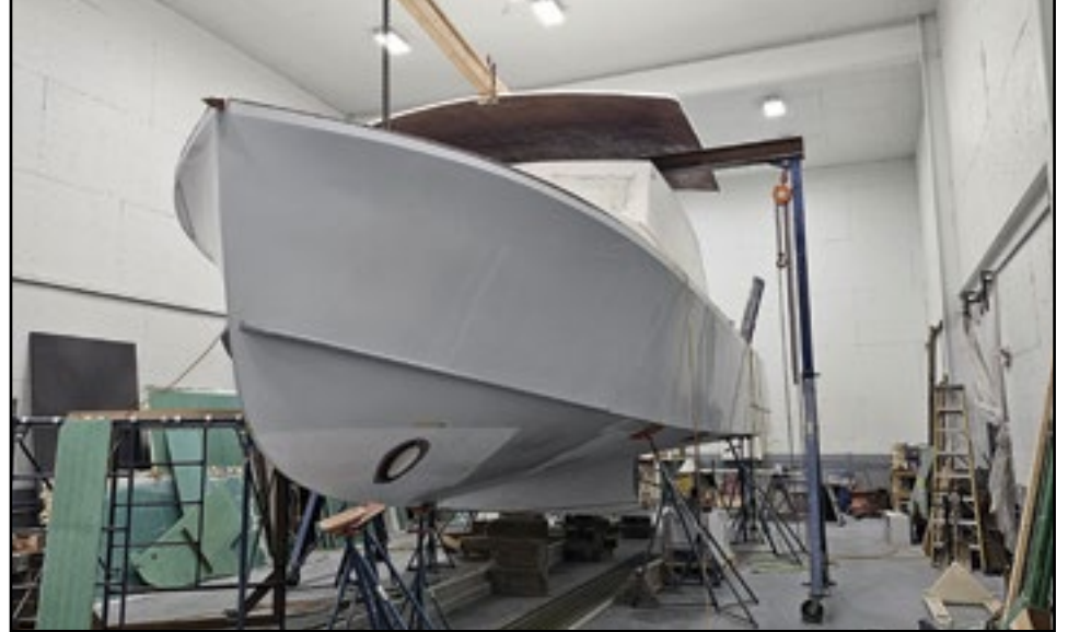
A Mussel Ridge 42 just being started at Samoset Boat Works in Boothbay. She will be finished out as a sportfisherman for a customer from Cape Cod. They are working on tankage under the platform and roughing in the interior.
