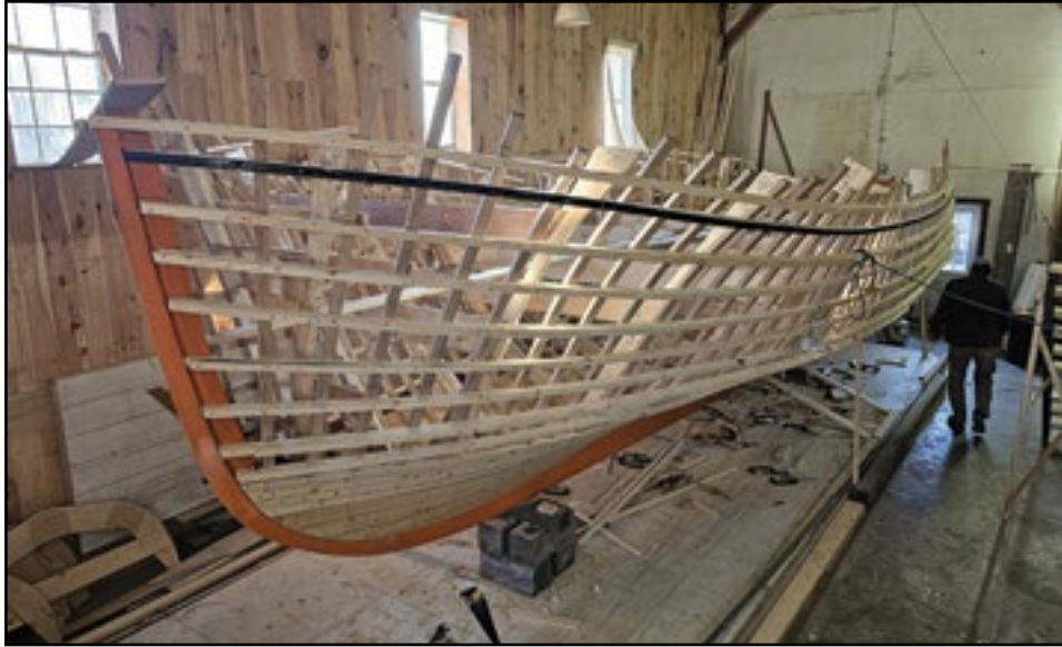
Peter Buxton of Buxton Boats in Sunset has the 32-footer all framed out and has started planking the bottom.
