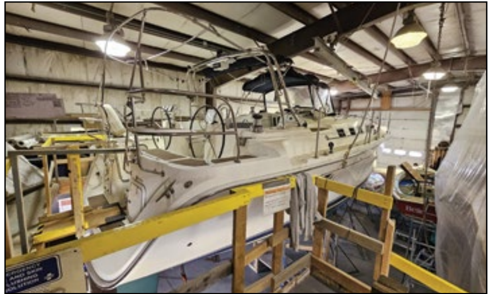
This is a Hunter 49 sailboat in at Johanson Boat Works in West Rockport. She has some minor damage to repair as well as replace generator, windows and electronics. Just to her side you can see one of the Camden Yacht Club’s launches, which is in for a new 50-hp Beta engine and fuel tank.
