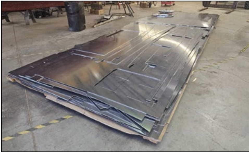
Believe it or not, this is a boat. Fogg Boat Works of North Yarmouth is working at a shop in Brunswick where they will be building two of their aluminum launches for a customer from out-of-state.
