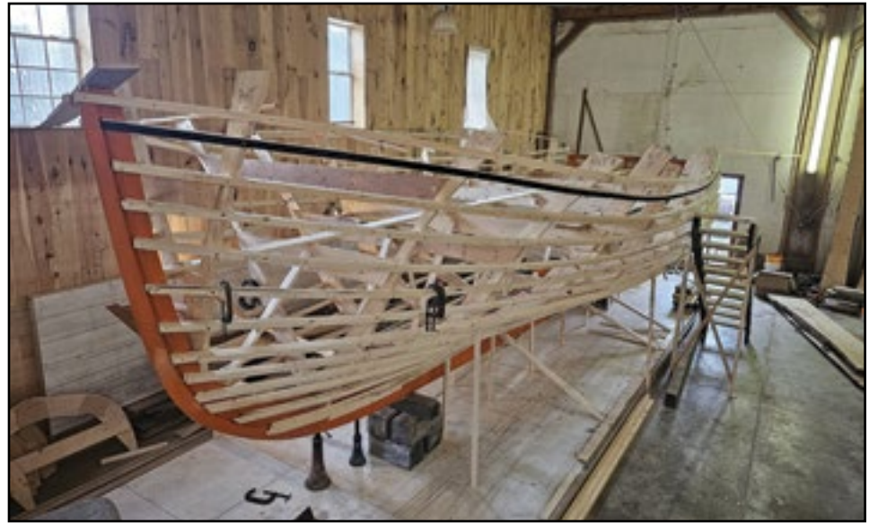
Peter Buxton of Buxton Boats in Sunset is getting ready to frame up this 31+-foot lobster boat hull. The steam box was releasing steam and soon the frames would be ready to go on.
