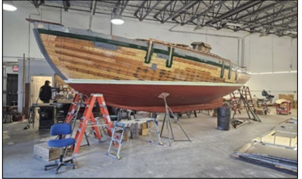
The Alden schooner being repaired by Richard Stanley and Sawyer Theriault at the owner's shop in Brunswick. The hull is done and they are now working on her interior.
