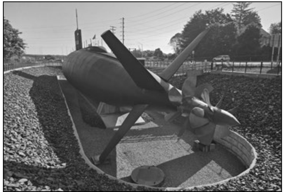
A stern view of USS ALBACORE showing her stern planes and her concentric contra rotating propellers.
