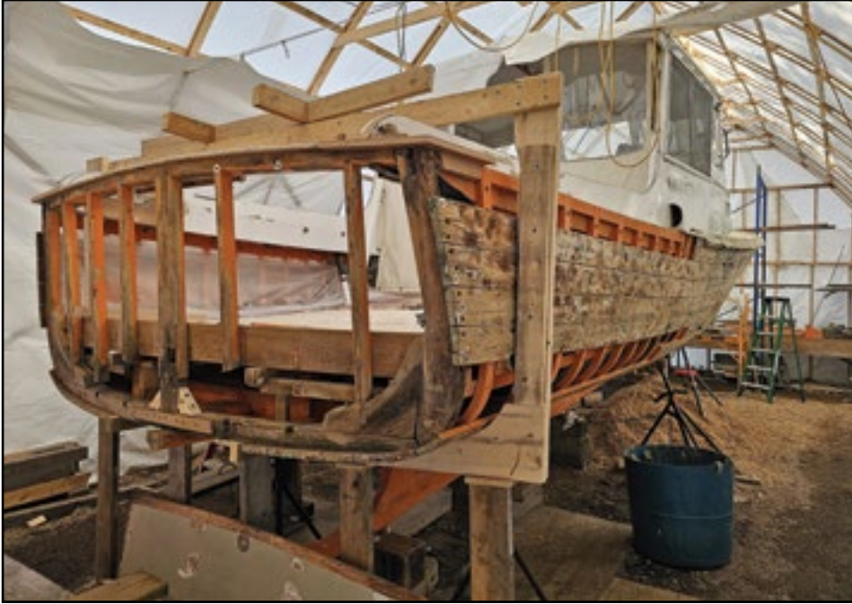
This is a view of the transom of HARPOON, being repaired by Downeast Custom Boats in Yarmouth. She was Lowell designed and built.
