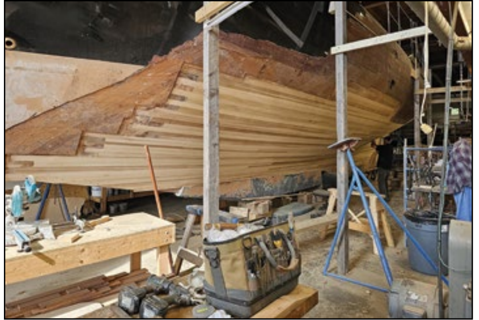
In the last issue of Maine Coastal News , I did a write up in Boat Yard News on Rockport Marine repairing a cold moulded sailboat, which had grounded in a storm in Narragansett Bay. She had numerous holes in her portside and they were made into one big hole. Here you can see that the big hole is now getting filled in with strip planks fore and aft, which is the first of four layers.
