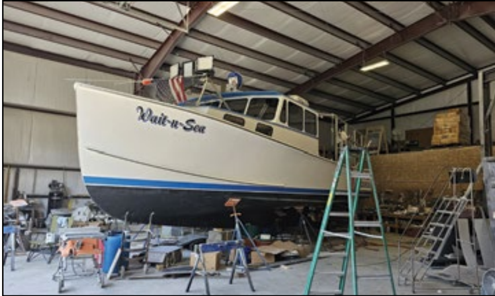
The 42-foot RP WAIT-N-SEA is in for major modifications at Friendship Boat Works in Friendship. They changed the transom and added a split wheelhouse.
