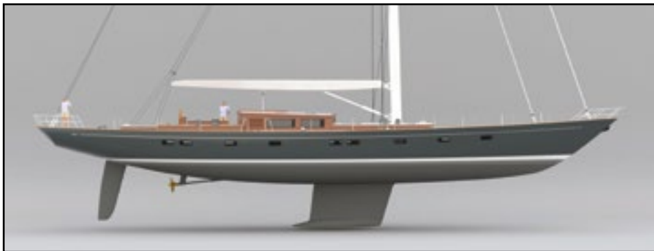
This 95-foot sailing yacht is now under construction at Rockport Marine in Rockport. The hull was built upside down and they are now fairing before she is rolled over. This boat is expected to be completed the summer of 2025.
