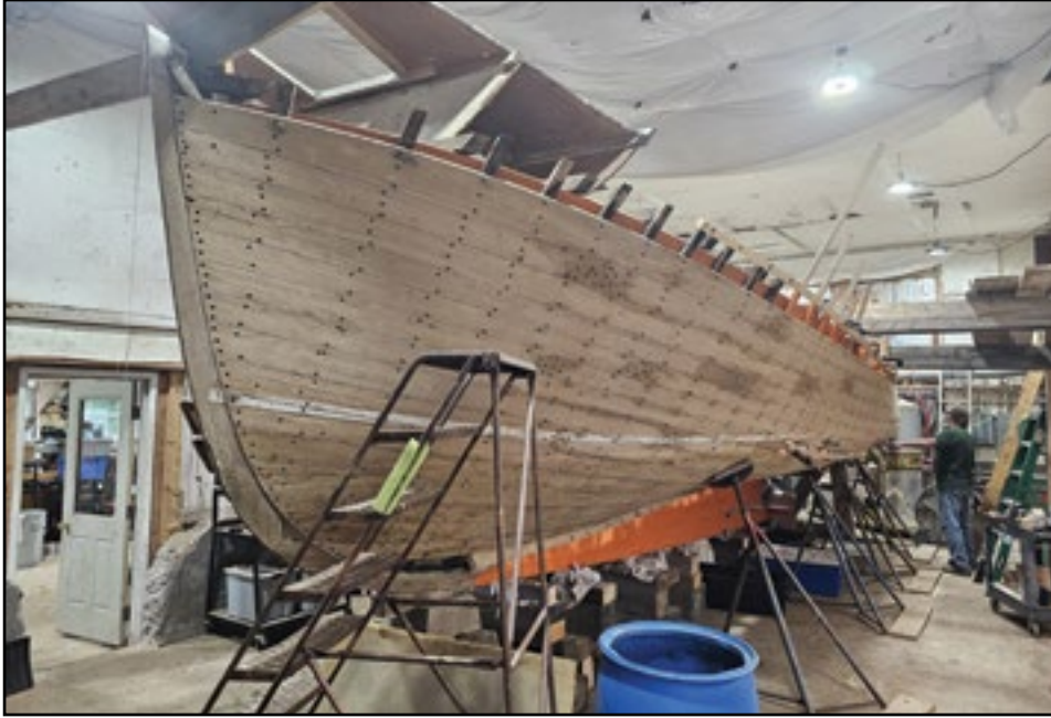
The lobster boat ROYAL with her new keel and about 40 frames in place at Downeast Custom Boats in Yarmouth. They are now getting ready to work on her bow frames and stem.
