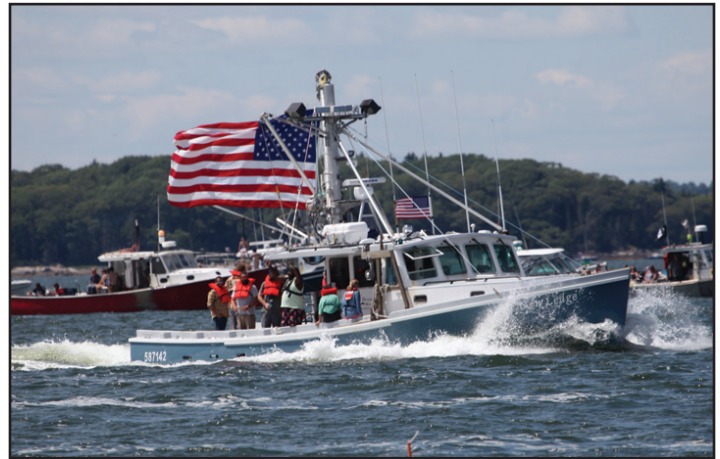
Parker Poole's NEW LEDGE [Stanley 44; 304-hp 871 Detroit] storming up the course for a fourth place finish at a speed of 10.8 mph.
