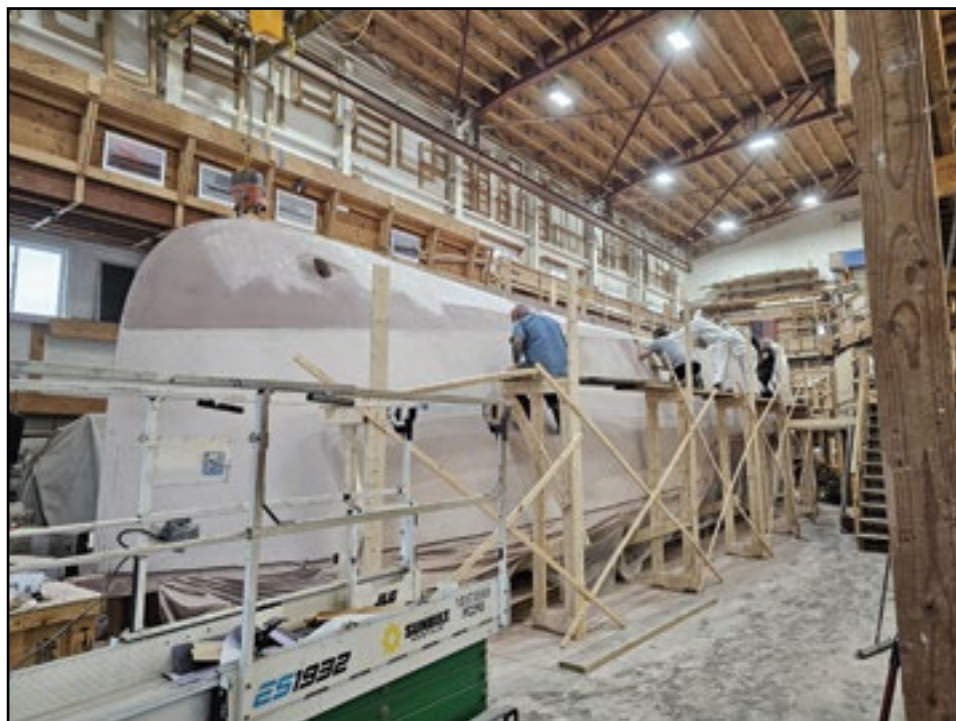
At Brooklin Boat Yard the cold moulded hull off the Wheeler 55 has been layered up and they are now long boarding to get her perfectly smooth.
