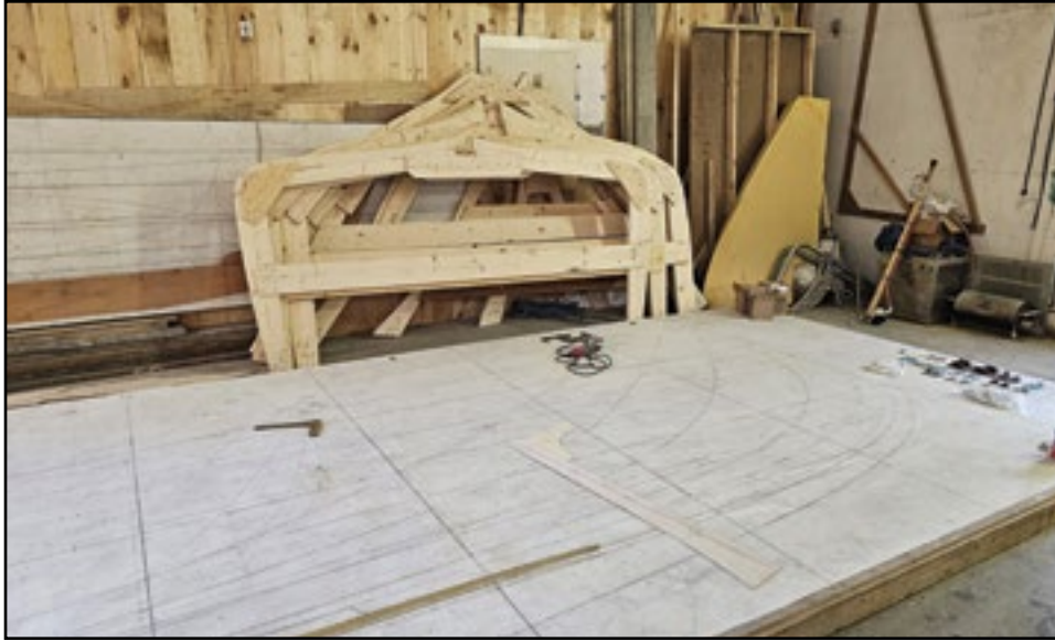
At Buxton Boats in Stonington, they have started building a 32+ foot wooden boat. You can see the lofting on the floor and the mould stations laying up against the wall.
