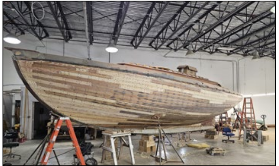
The Alden schooner being rebuilt by Richard Stanley and Sawyer Theriault in Brunswick. They were caulking and putting in seam compound and next they would be fairing.
