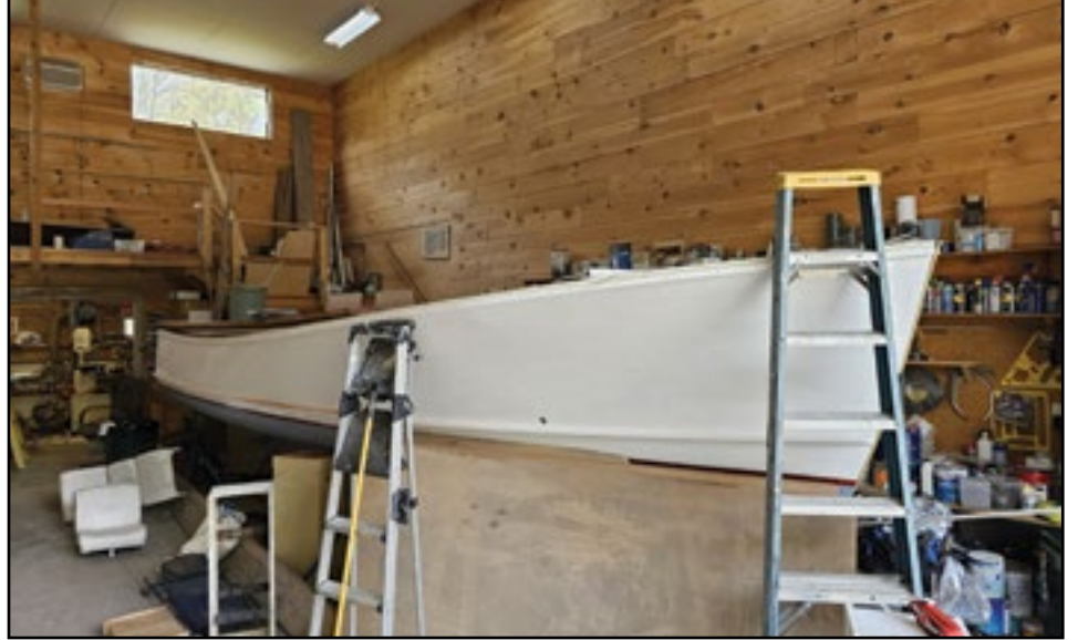
The Hodgdon 24 hull, which has been rebuilt by Shop to Shore for a customer who lost his boat to a fire. She will go out as a centre console.
