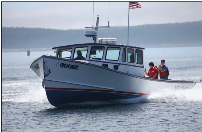
The only entrant in Diesel Class J was Carroll Staples' GOOSE [Mitchell Cove 37; 650-hp Volvo].
