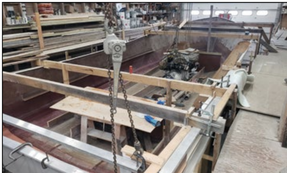
This is a Young Brothers 40 hull, which has been lengthened and widened at Little River Boat Shop in Cutler. Ryan Lemieux said it took them a little more than a week to do.
