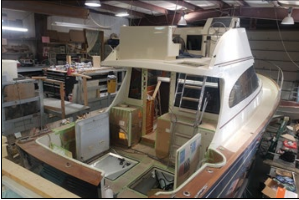
This is a York 42 of Northeast Harbor, which has been in the shop for a major overhaul by York Marine of Rockland. They made modifications to the flybridge, repowered and made modifications to the interior. She is close to being finished and should be over mid-spring.
