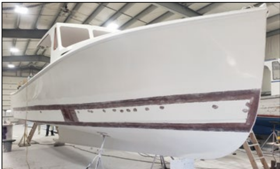
At Wayne Beal's Boat Shop in Jonesport they are finishing up putting the hard chines on another Wayne Beal 36. She is being finished out for a customer from Martha's Vineyard.
