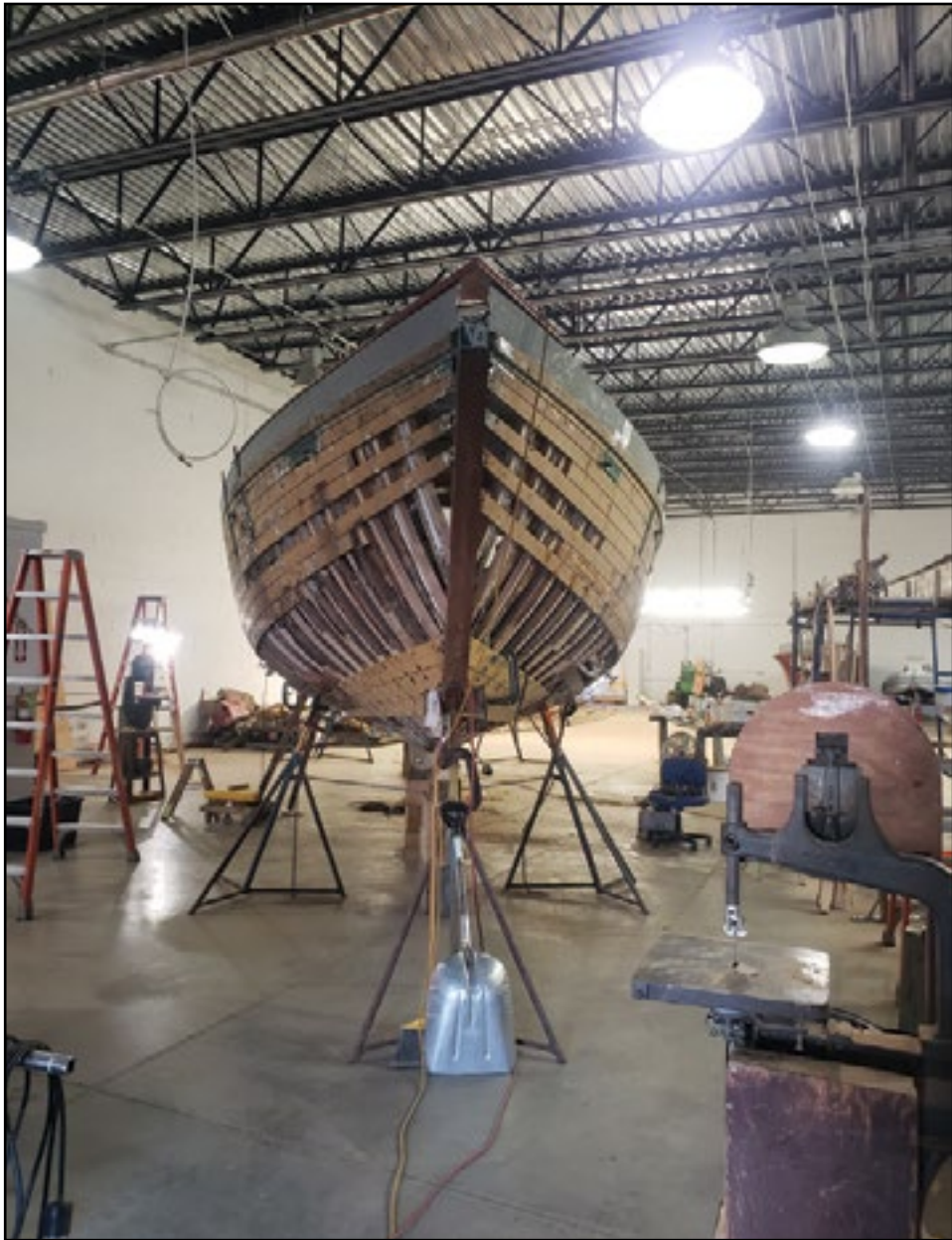
A bow view of the Alden schooner Richard Stanley is rebuilding in Brunswick for her owner. He at first did not think she was a good-looking boat, but he has changed his mind. He, along with an assistant, are now replacing a number of frames.
