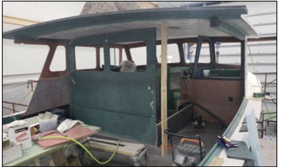
This is a Mussel Ridge 42 split wheelhouse lobster boat being finished out at Samoset Boat Works in Boothbay for a fisherman from Sedgwick.
