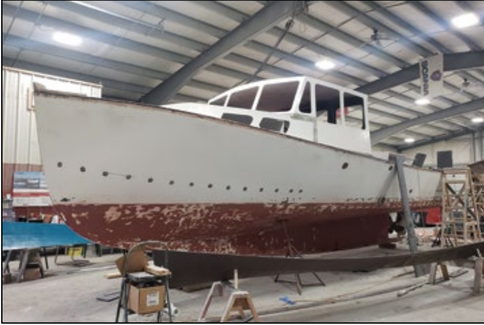
At Wayne Beal Boat Shop in Jonesport, they have this Young Brothers 38 getting totally refurbished. They have put one of their tops on and have much of the internal structure completed. She will also be fitted with hard chines before going out later this fall.
