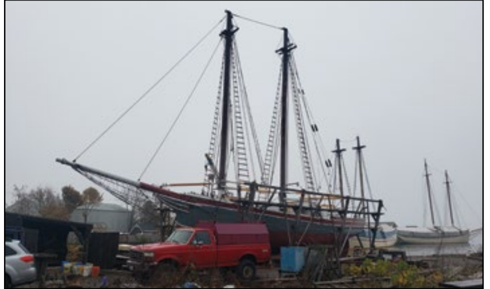
The schooner LEWIS R. FRENCH hauled up on the ways at Northend Shipyard in Rockland. She had a few planks replaced and paint.
